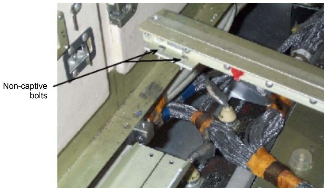
Figure 12.1-2. Transverse Tee Bracket to be removed during Storage Battery A73 Changeout (a close view with both nuts already removed)
