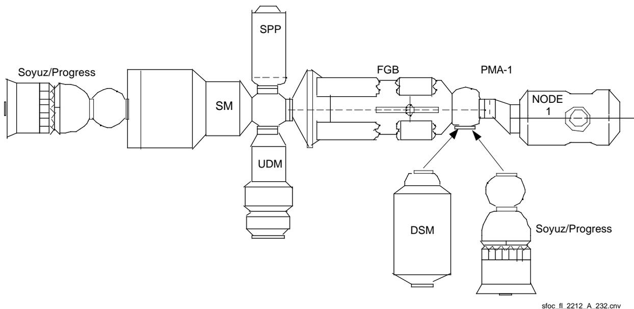
**Figure 1-1. Assembly of the International Space Station**
