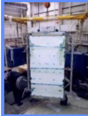
Early External Active Thermal Control System (EEATCS) (Boeing Canoga Park) [S/C - Lockheed Vought]
