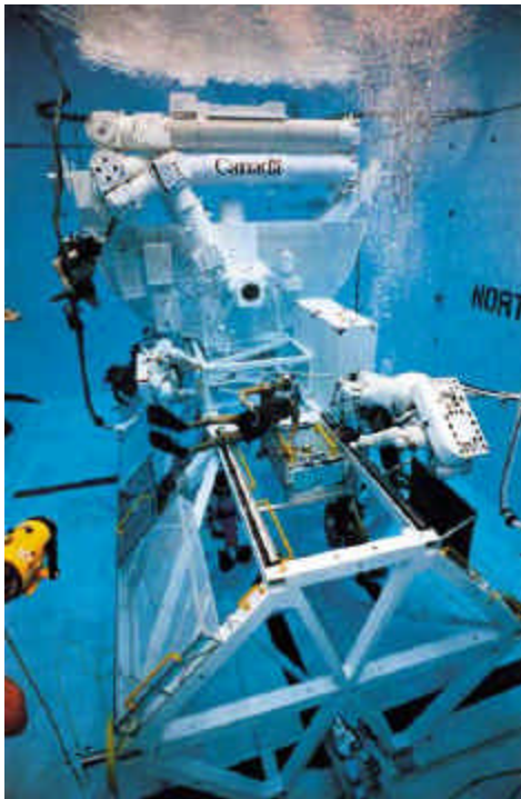
Testing the SSRMS in the Neutral Buoyancy Lab at the Johnson Space Center
