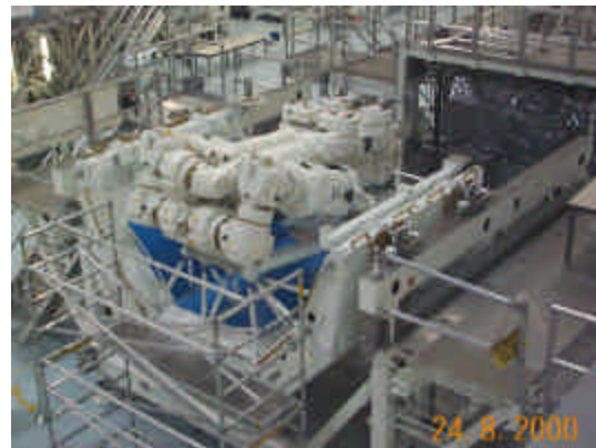
The SSRMS on its pallet awaiting its launch in April 2001
