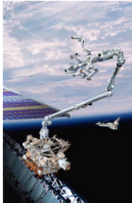
This 17-metre, 1,5-ton arm is essential to the construction of the ISS, to many Station operations and to the maintenance of the Station throughout its service life.
